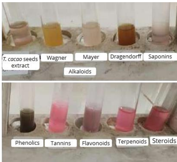
Figure 1. Photographed images of T. cacao seeds extract before and after the phytochemical test.
